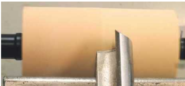
▲ Pic.6 Using the centre for the initial cutting allows the wings of the tool to remain sharp. You can now utilise these for your finishing cuts
